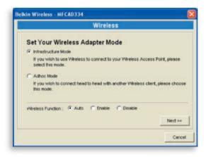
Double-click the "Wireless" icon and the "Wireless" configuration window pops up. If you use an access point to build up your wireless network, you have to select "Infrastructure Mode". If you do not have an access point and want to use a peer-to-peer connection to build up your wireless network, you have to select "Ad-Hoc Mode". After selecting the operation modes of the wireless function, click "Next" to go to further detailed configuration.
